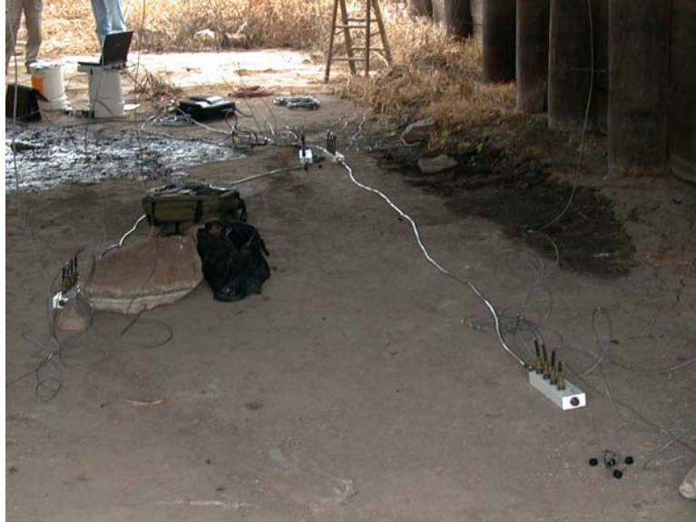
Figure 4.4. BDI STS Units in use during a load test.
