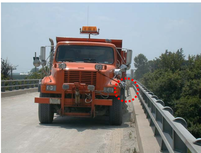
Figure 4.6. BDI Autoclicker in use during a load test.
